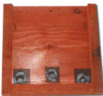
1. Take a 15x15 piece of redwood framed with 2x2's on three sides. Add three holes for drainage with screen to keep out bugs
